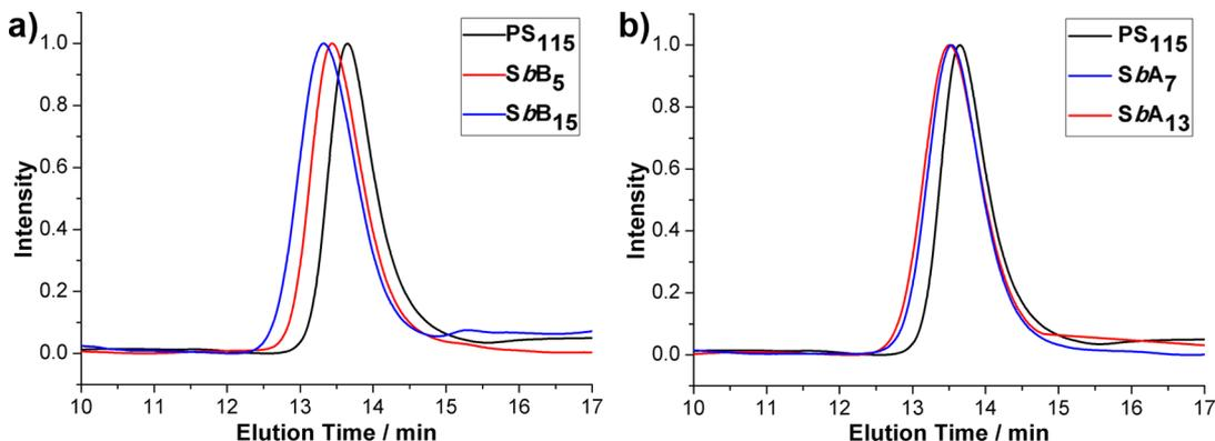
**Figure 2.** GPC curves of (a) *SbB*<sub>5</sub>, *SbB*<sub>15</sub> and (b) *SbA*<sub>7</sub>, *SbA*<sub>13</sub> and the corresponding macro-CTA *PS*<sub>115</sub> in DMF.
