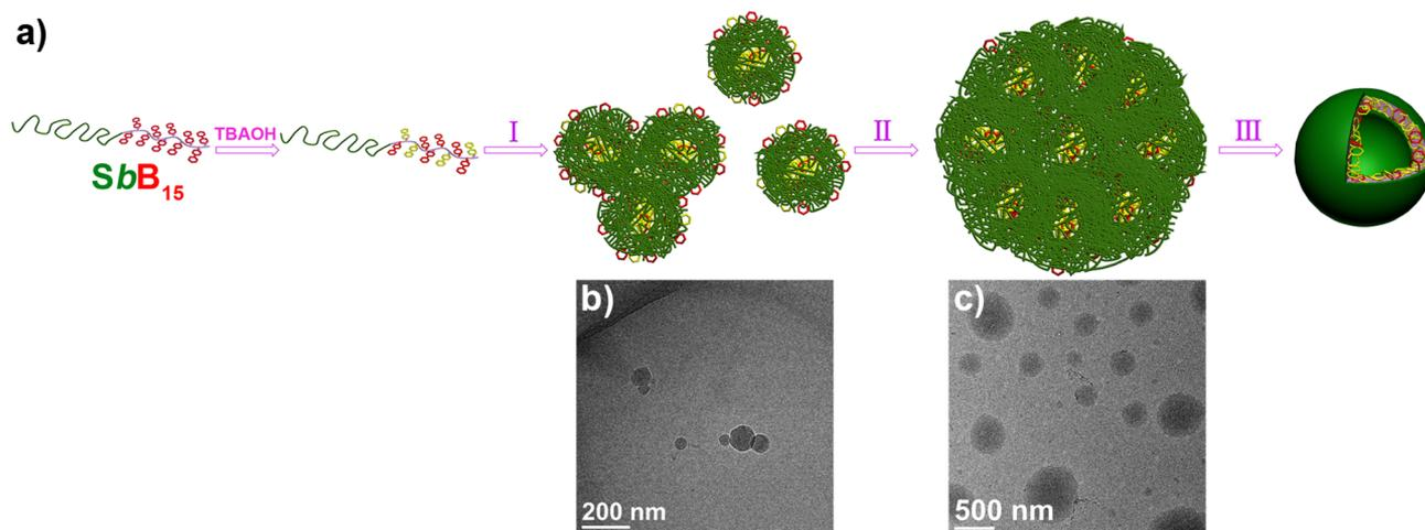
**Figure 8.** (a) Proposed mechanism of the assembly process in Figure 7a. Cryo-TEM images of the assemblies collected at (b) state I and (c) state II as arrowed in Figure 7a.
