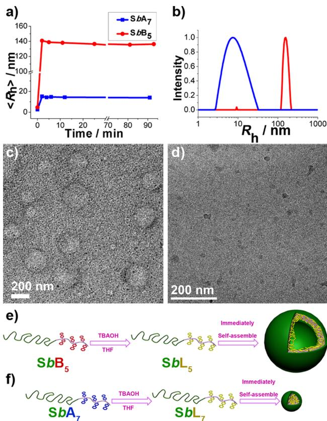
**Figure 5.** (a) Evolution of  $\langle R_h \rangle$  during the self-assembly process started from addition of TBAOH (13.3  $\mu$ L, 4.0 equiv) into the solution of  $SbB_5$  and  $SbA_7$  (1.5 mL, 1.25 mg/mL) in THF. (b)  $R_h$  distribution of  $V-Bz-4$  and  $M-Ac-4$ . The cryo-TEM images of (c)  $V-Bz-4$  and (d)  $M-Ac-4$ . Cartoon scheme of self-assembly of (e)  $SbB_5$  and (f)  $SbA_7$ .
