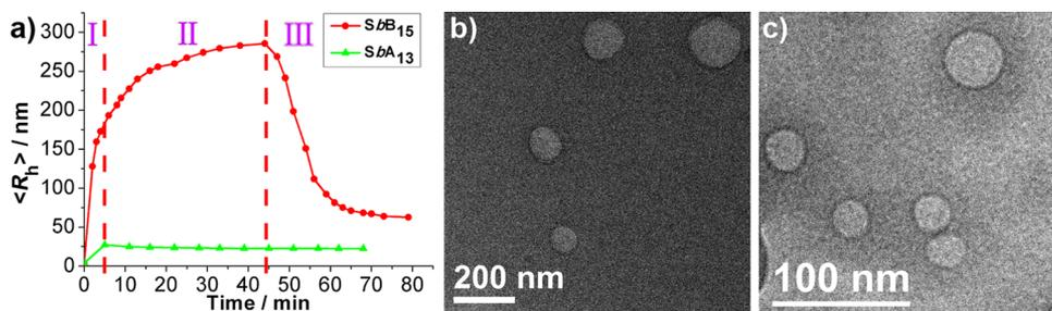
**Figure 6.** (a) Evolution of  $\langle R_h \rangle$  during the self-assembly process starting from addition of 8.0  $\mu$ L of TBAOH (1.0 equiv) into the THF solution of  $SbB_{15}$  (red line) and  $SbA_{13}$  (green line) (1.5 mL, 1.25 mg/mL). The cryo-TEM images of (b)  $V-Bz-5$  and (c)  $V-Ac-5$ .
