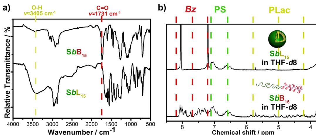
Figure 3. (a) FT-IR spectra and (b)  $^1\text{H}$  NMR of **SbB<sub>15</sub>** and **SbL<sub>15</sub>**. For FT-IR, after 10 min reaction and dialysis against water, the resultant powder of the deprotected product was collected and used for the measurement.
