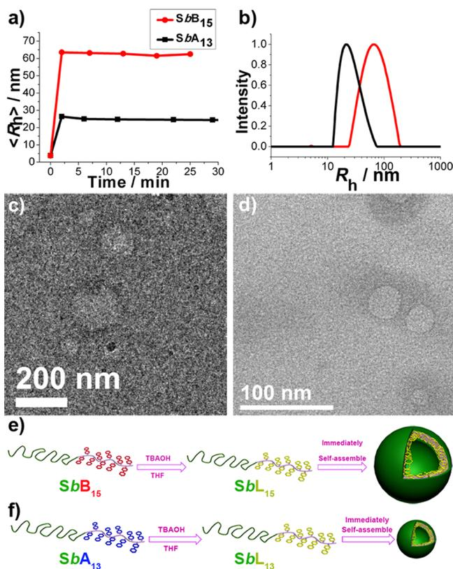
**Figure 4.** (a) Evolution of  $\langle R_h \rangle$  during the self-assembly process started from addition of excess amount of TBAOH (40 wt %, 10  $\mu$ L) into the THF solution of  $SbB_{15}$  and  $SbA_{13}$  (1.5 mL, 1.25 mg/mL). (b)  $R_h$  distribution of  $V-Bz-3$  and  $V-Ac-3$ . Cryo-TEM images of (c)  $V-Bz-3$  and (d)  $V-Ac-3$ . Cartoon scheme of self-assembly of (e)  $SbB_{15}$  and (f)  $SbA_{13}$ .
