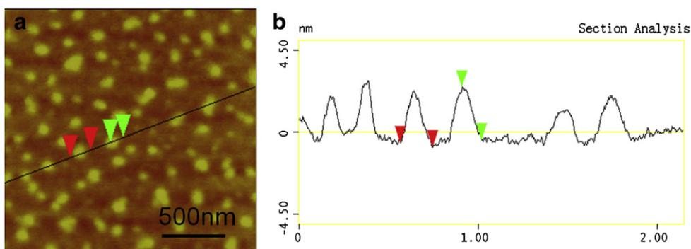
**Fig. 2.** (a) AFM image of vesicles formed while  $C_{12}$ -PNIPAM-CA in deionized water (0.1 mg/mL) was kept at 35 °C for 30 min before dripping onto mica; (b) section analysis of the image with horizontal distance of 184 nm (red arrows) and vertical distance of 3 nm (green arrows). (For interpretation of the references to colour in this figure legend, the reader is referred to the web version of this article.)
