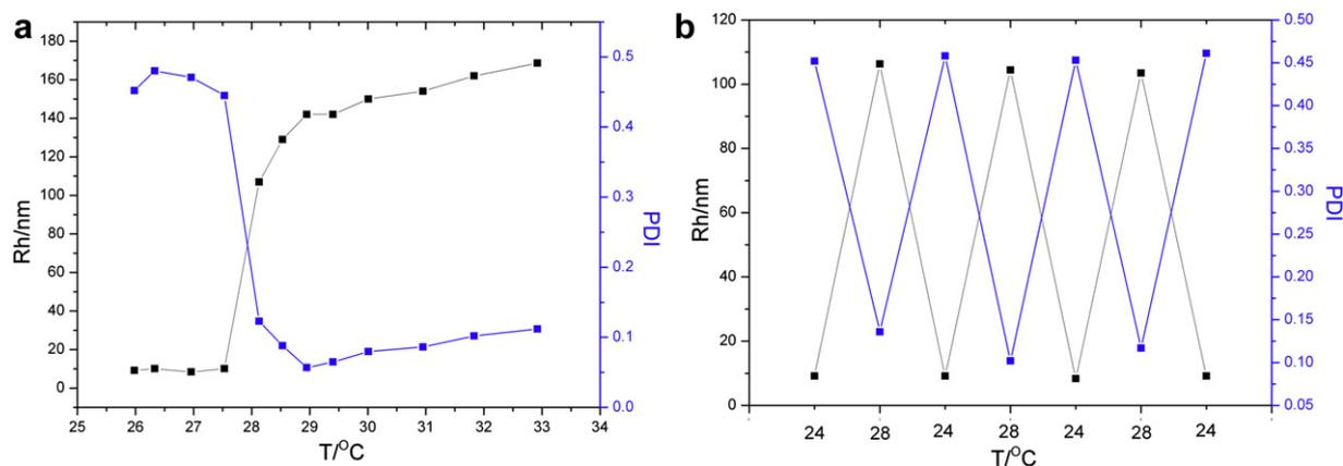
Fig. 8. Light scattering study of 0.1 mg/mL  $C_{12}$ -PNIPAM-BA in water: (a)  $R_h$  and PDI recorded after 30 min heating at a given temperature, (b) morphology transition cycles between 24 °C and 28 °C.
