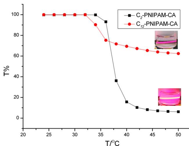
**Fig. 4.** Transmittance at different temperatures and photos taken at 45 °C of  $C_{12}$ -PNIPAM-CA and  $C_2$ -PNIPAM-CA in deionized water at the concentration of 0.2 mg/mL.
