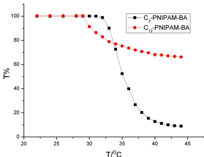
Fig. 7. Transmittance of  $C_{12}$ -PNIPAM-BA (0.2 mg/mL) and  $C_2$ -PNIPAM-BA (0.2 mg/mL) at different temperatures.
